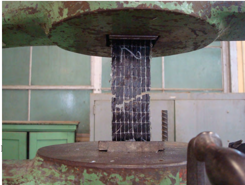
Figure E.7 Rupture of the coupon
