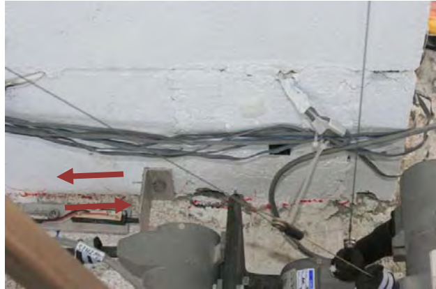
Figure 6.12 Sliding in W-2 after 100% Chi Chi event (Stavridis)
