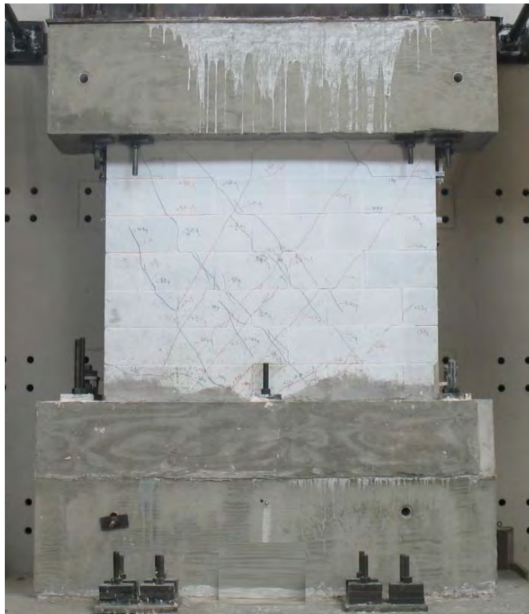
Figure 6.41 Masonry wall with concrete ring applied.
