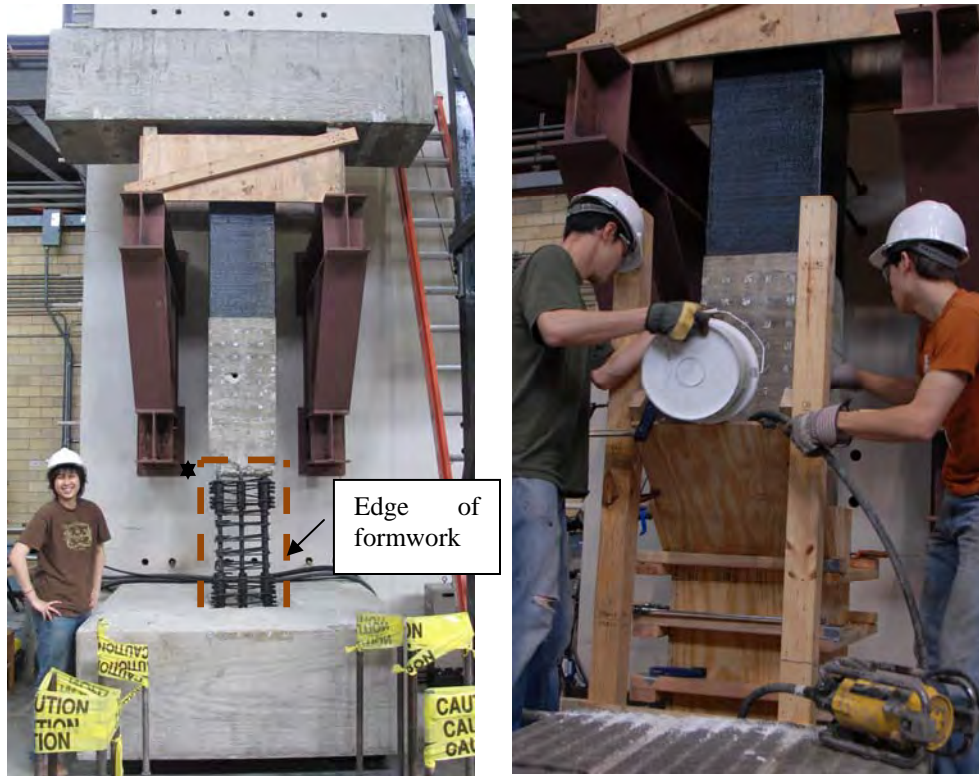
Figure 5.49 Column with the Mechanical Splices Applied (left) and placement of concrete (right)
