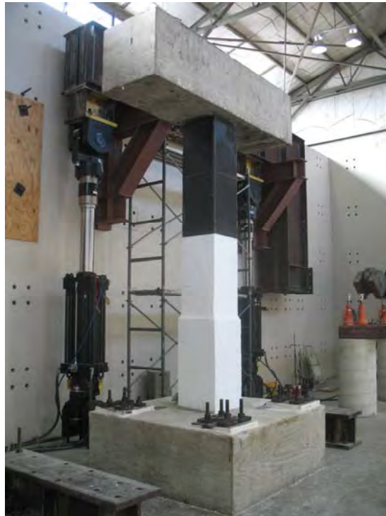
Figure 1.7 Column damaged retrofitted by CFRP jacketing and mechanical splices
