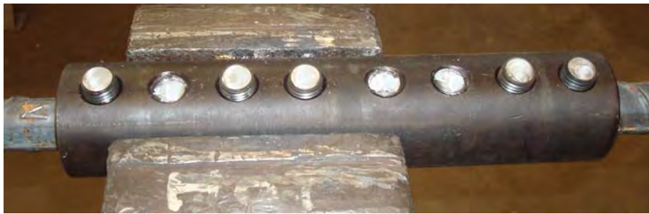
Figure I.30 Condition of MS-L3 after the tightening
