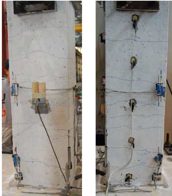
Figure 5.103 Propagation of cracks on north (left) and south (right) face of the specimen at yielding (1.05% drift ratio)
