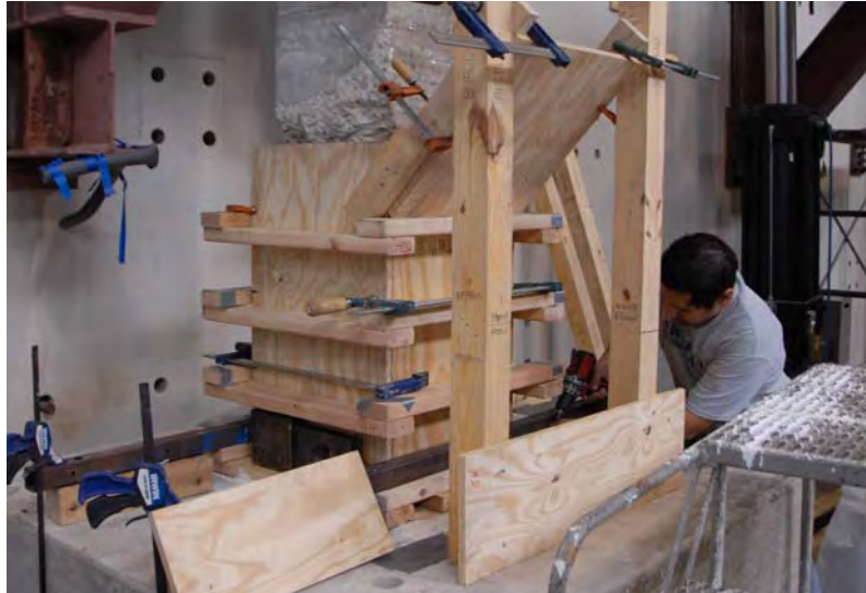
Figure B.17 Form for the casting of concrete in bottom of column
