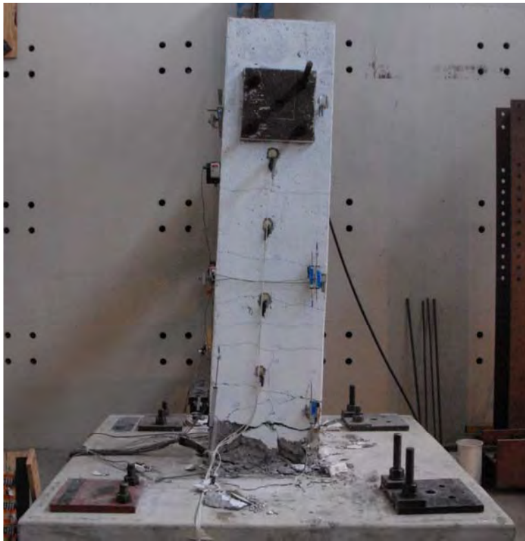
Figure 5.109 Specimen twisting at the base before rupture of NW existing bar. The column is inclined to the south-west corner since only NW bar is carrying tension.
