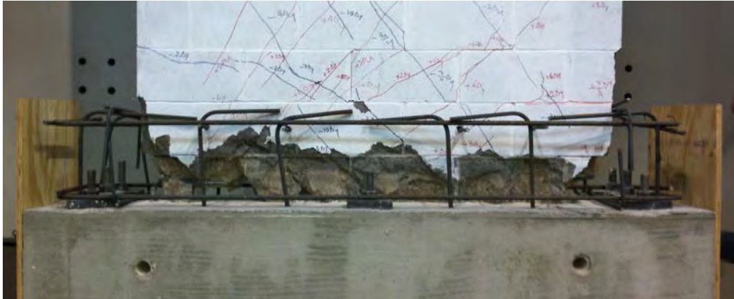
Figure D.2 Installation of the reinforcement for the concrete ring (RMW-R1)
