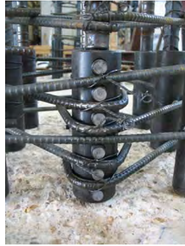
Figure 5.90 Short mechanical splices completely installed for specimen RC-2R-SMS
