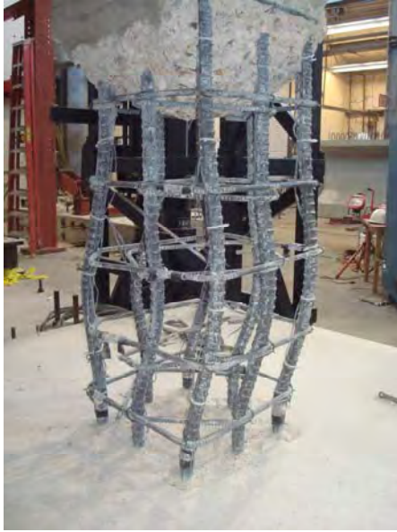
Figure B.12 Buckled bars and opened ties in bottom of column (left) and removing of the damaged bars (right)
