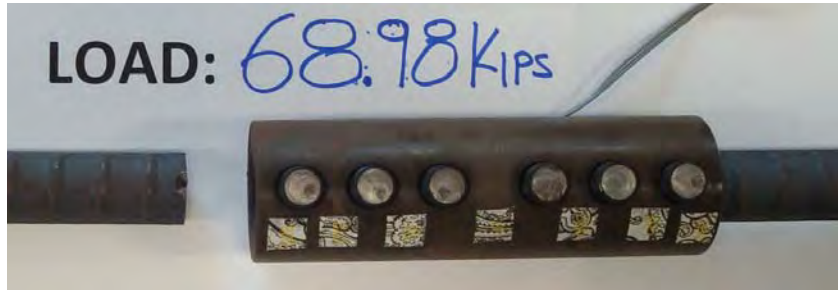
Figure I.12 Specimen MS-S1 after failure
