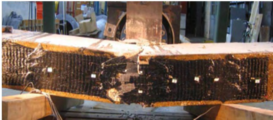
Figure 4.2 CFRP sheet rupture when anchor used. (Kim 2006.)
