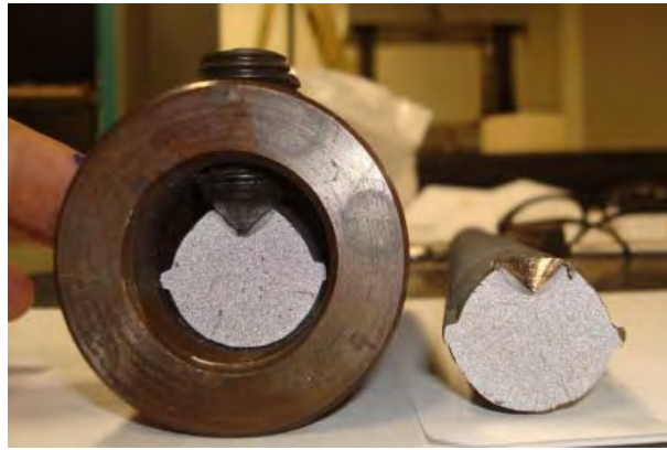
Figure I.22 Cross section of the bar broken of MS-S2
