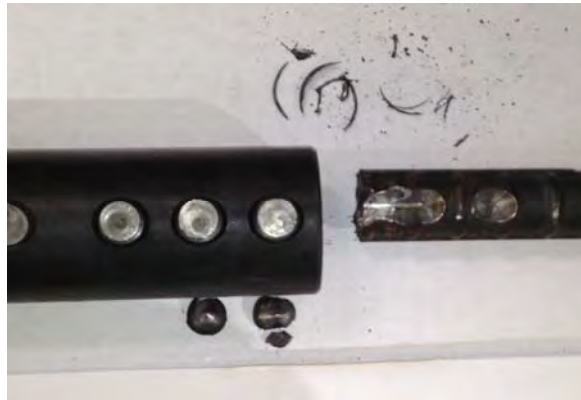
Figure I.67 Bolts broken on the thread between the internal surface of the splice and the new steel bar.
