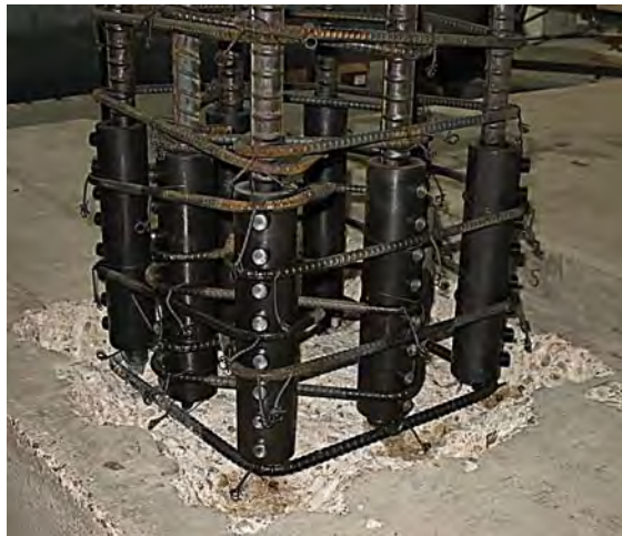
Figure 5.91 Long mechanical splices completely installed for specimen RC-2R-LMS
