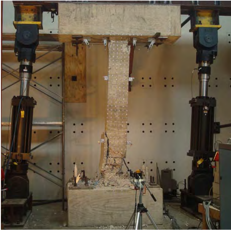
Figure 5.18 RC-1 at 19 th cycle loading to south. Spalling of the cover at top of column. Concrete crushing and buckled bars at bottom of column.
