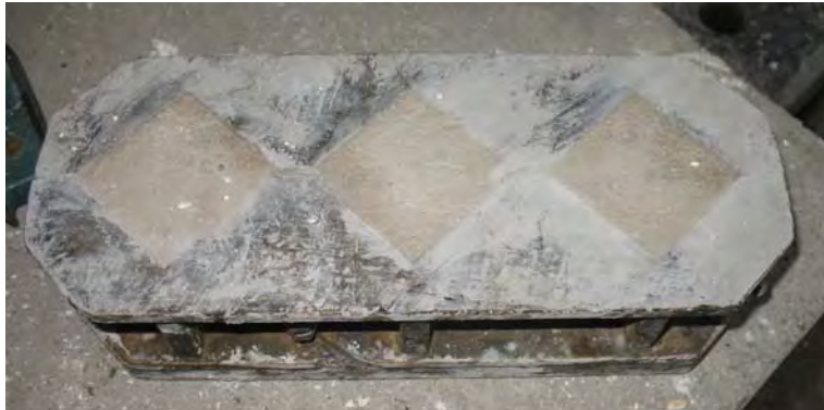
Figure E.8 Mortar cubes for compressive test
