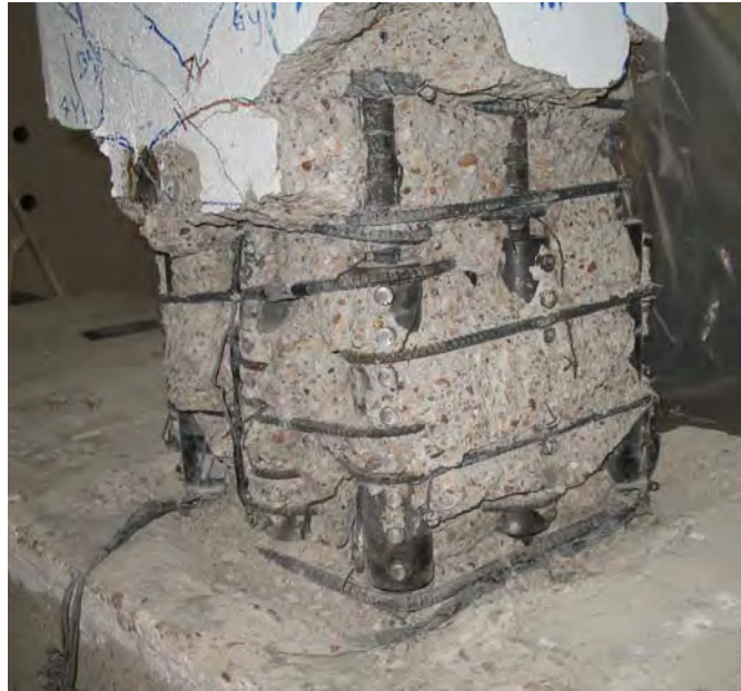
Figure 5.142 Final condition of the specimen after the test showing well-confined core.
