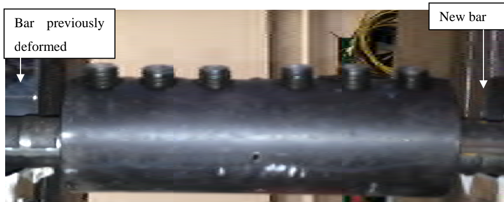
Figure I.52 No bolt broken on its thread area in specimen MS-S4
