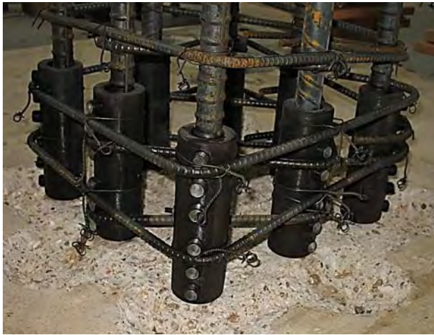
Figure 5.90 Short mechanical splices completely installed for specimen RC-2R-SMS
