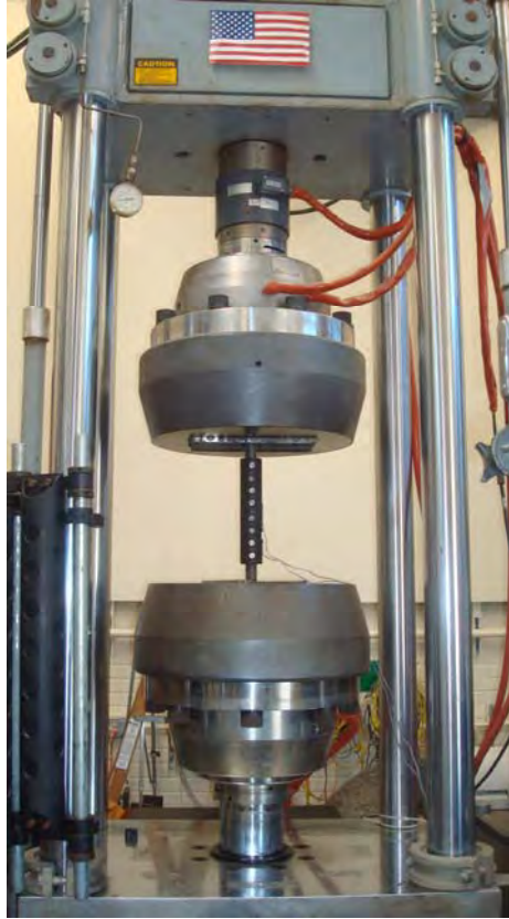
Figure 3.27 Test Setup for the compression-tension cycle test and details of the mechanical splices tested
