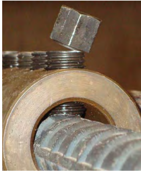
Figure I.41 Bolt's head removed from the edge of the thread
