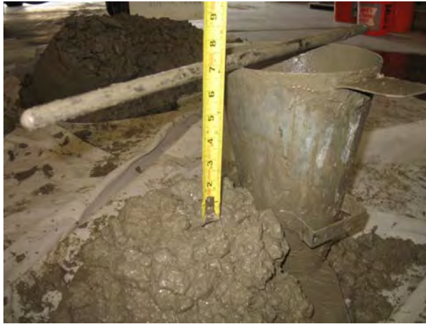
Figure D.4 Concrete placement, slump: 6.5in
