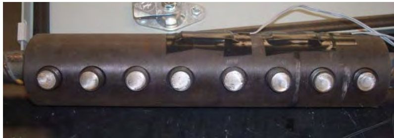
Figure I.42 Bolts of MS-L4 applied with shear cutting on the thread
