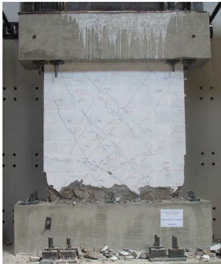
Figure D.1 Condition of RMW after initial tests
