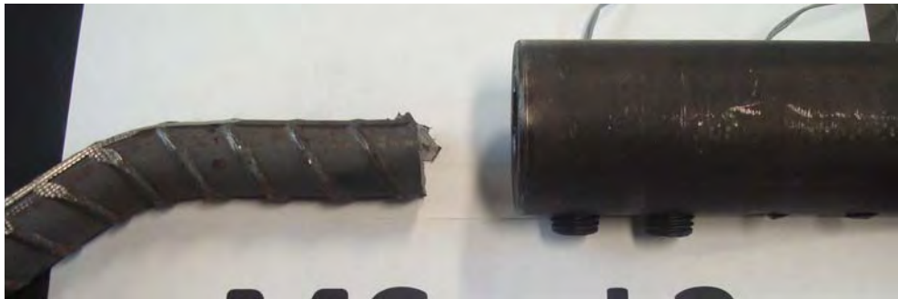
Figure I.36 Failure pattern, rupture of the bar of MS-L3
