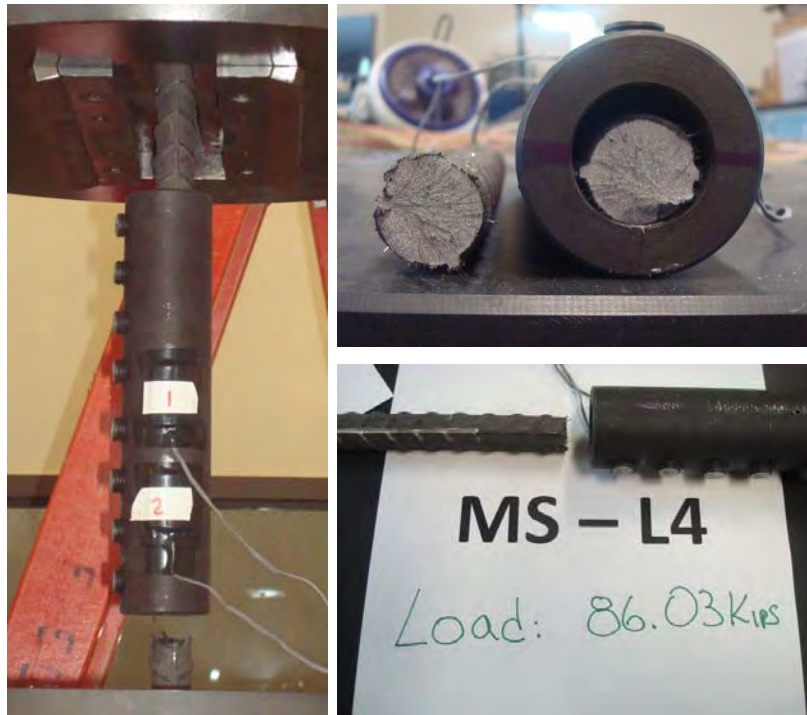
Figure I.46 Failure pattern for MS-L4
