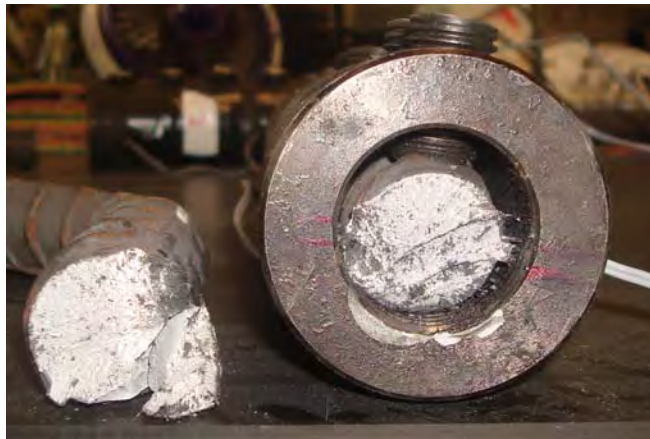
Figure I.37 Bar broken in the contact zone of rounded point bolt for MS-L3
