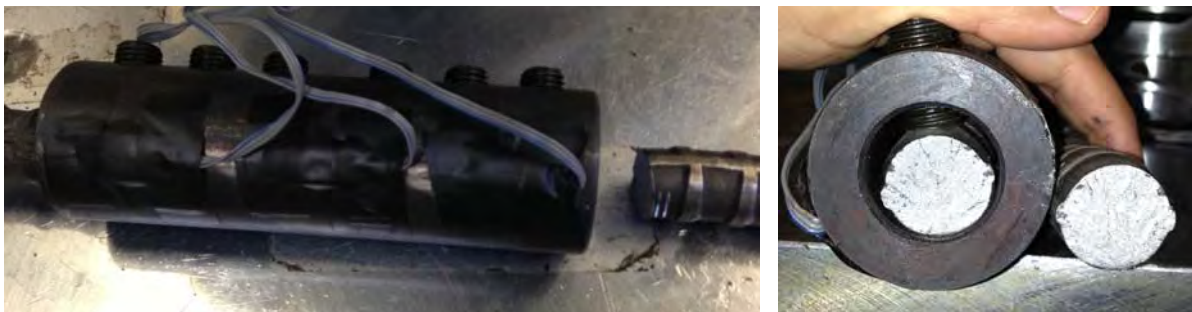
Figure 3.34 Failure under tension load: previously bar yielded was fractured
