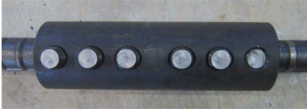
Figure 3.15 Head of the bolt broken
