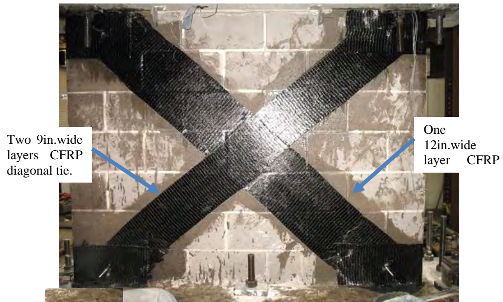
Figure 6.58 Back view (East side) of the masonry wall retrofitted
