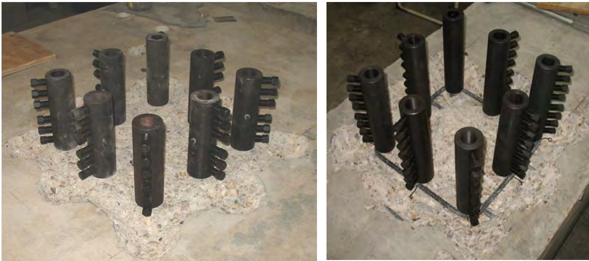
Figure C.5 Short (left) and long (right) mechanical splices in place.
