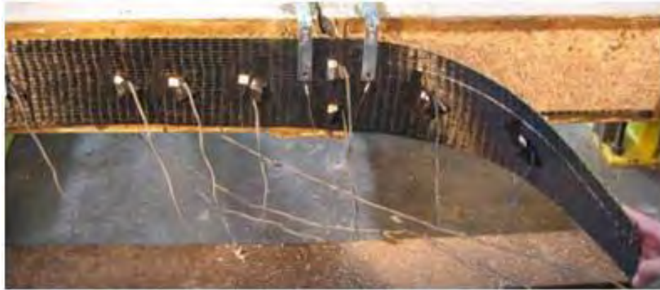
Figure 4.1 Debonding of CFRP sheet before strength of sheet is reached (Kim 2006)
