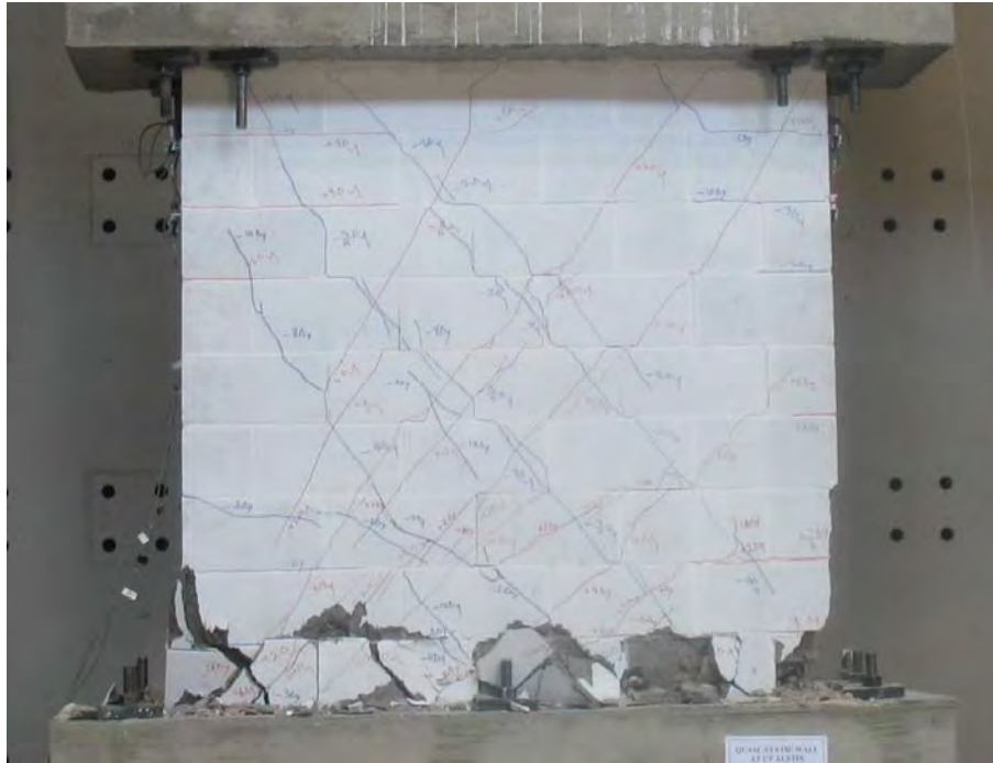
Figure 6.30 Crushing of masonry wall at end of the test
