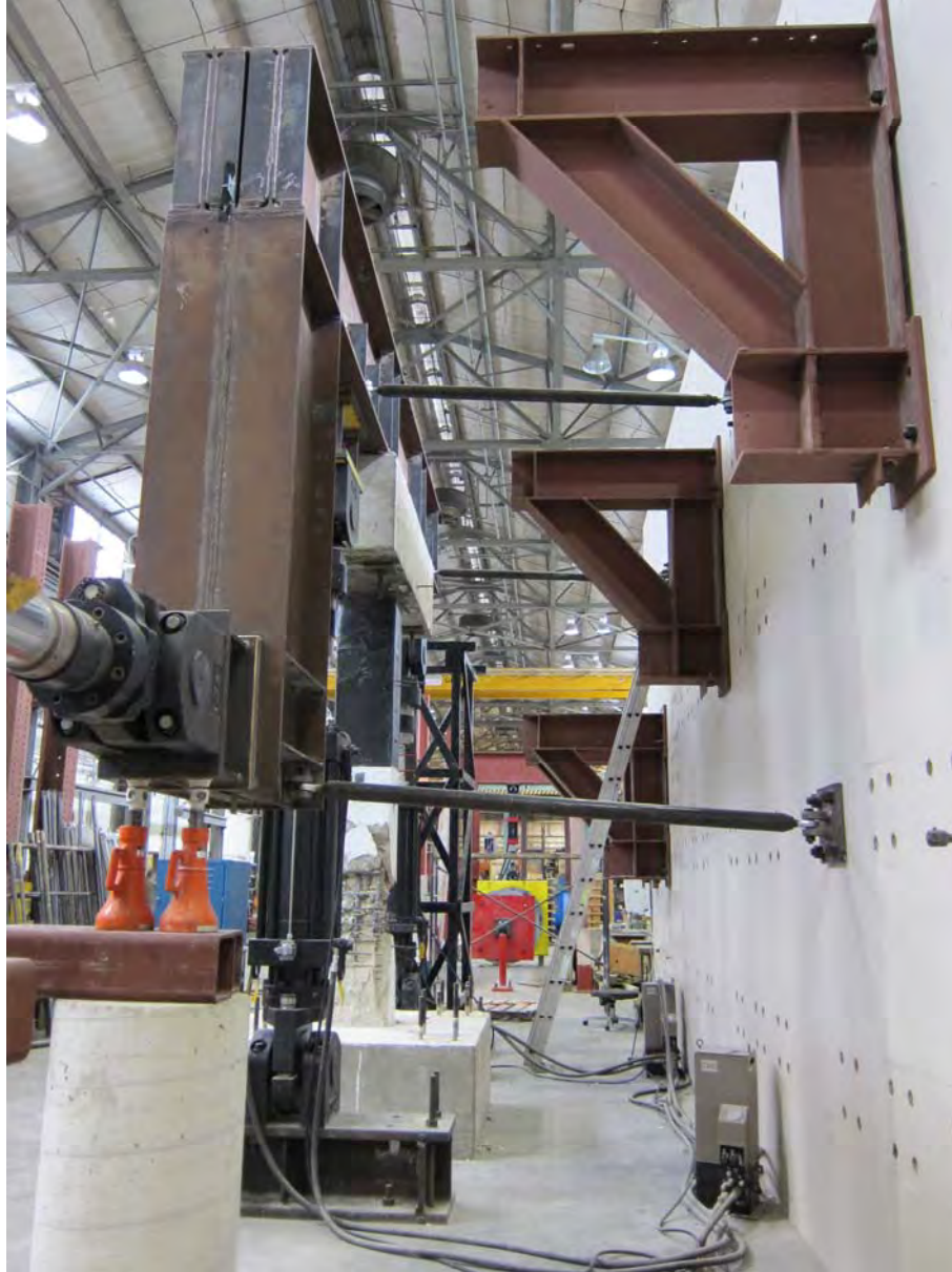
Figure F.2 Lateral braces to prevent the out-of-plane deformation and stabilization of L-frame setup
