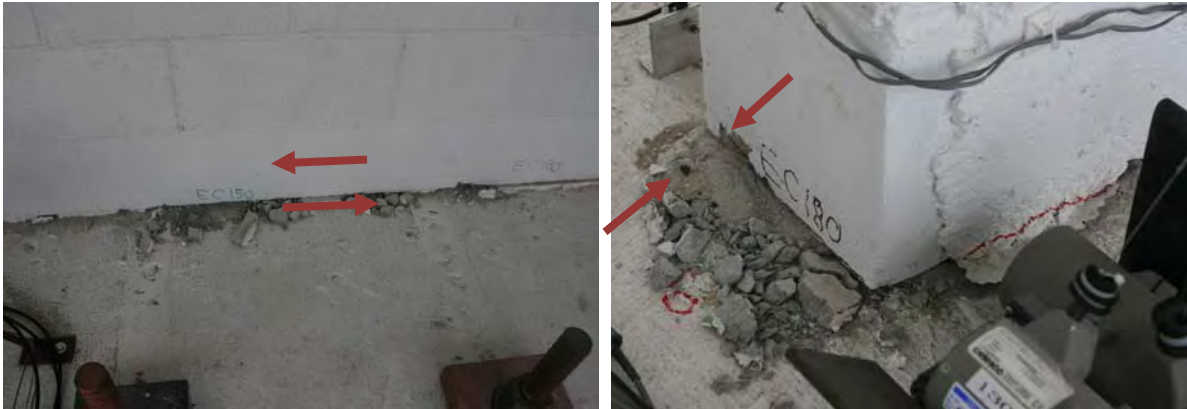
Figure 6.16 Sliding in W-2 after 2 nd 150% Chi Chi motion (Stavridis, 2011)
