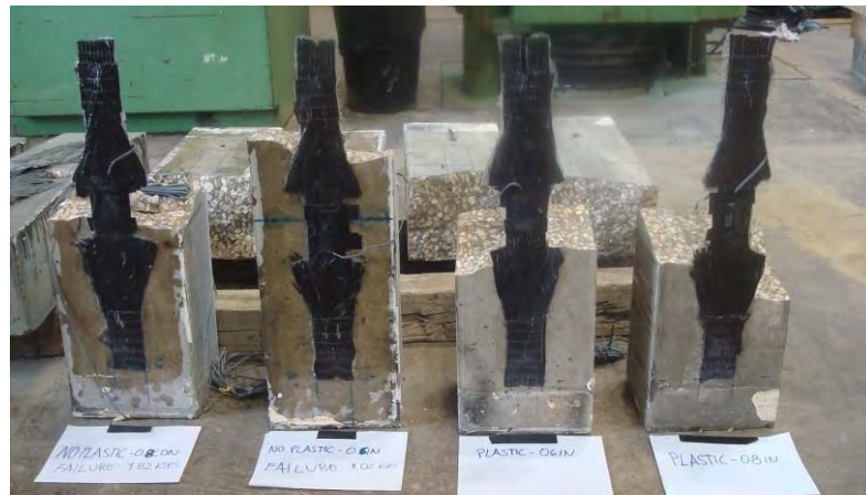
Figure 4.17 Fracture of CFRP anchors in all 4 tests
