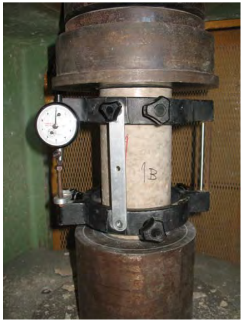
Figure E.2 Compressive test of concrete cylinder in universal machine
