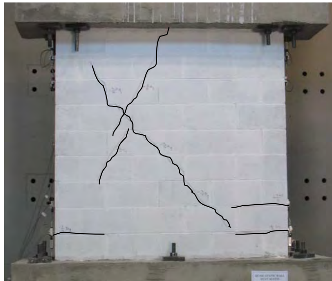
Figure 6.26 Horizontal, flexural and diagonal shear cracks
