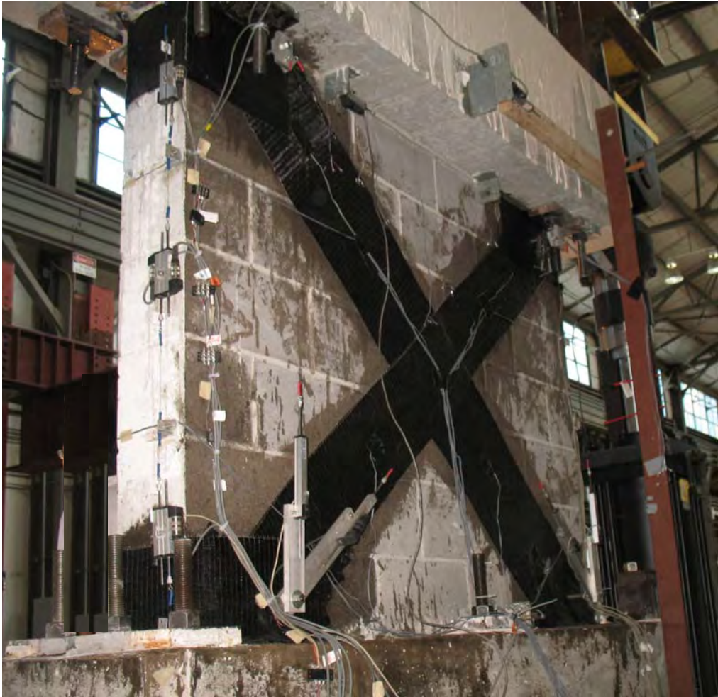
Figure 6.61 Linear potentiometer for local and global deformation measurement
