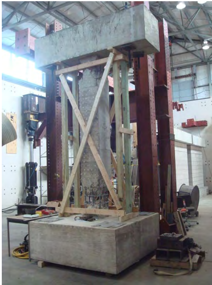
Figure C.1 Severely damaged column RC-2 removed from the test setup
