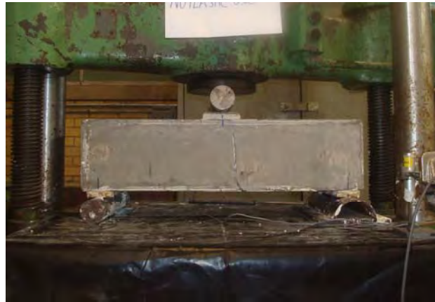
Figure 4.14 Specimen in test machine (test setup)
