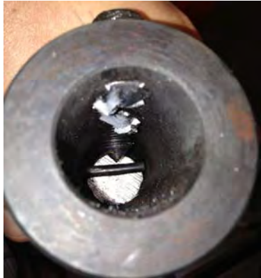
Figure I.67 Bolts broken on the thread between the internal surface of the splice and the new steel bar.
