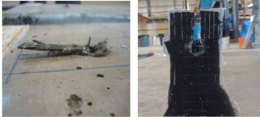
Figure 4.16 CFRP anchor fracture with unbonded sheets (Huaco, 2009)
