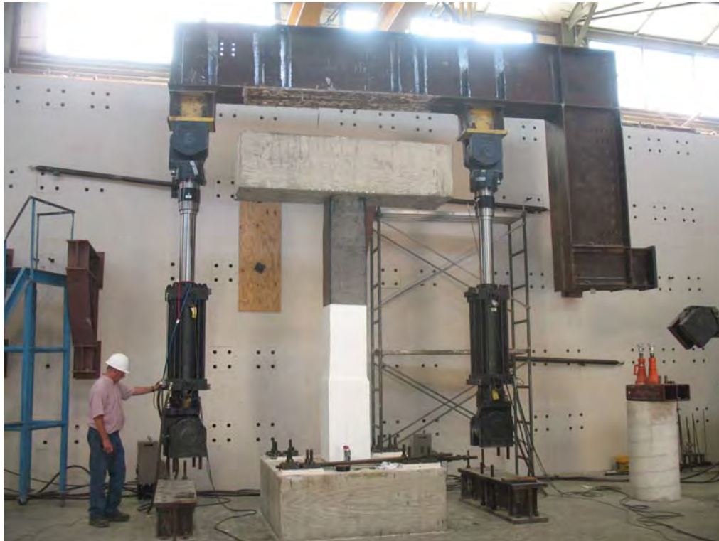
Figure F.1 Placement of L-frame setup on specimen RC-1R
