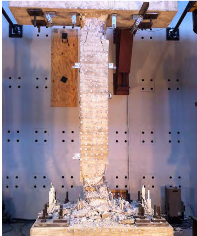
Figure 5.28 Condition of the column at the failure.
