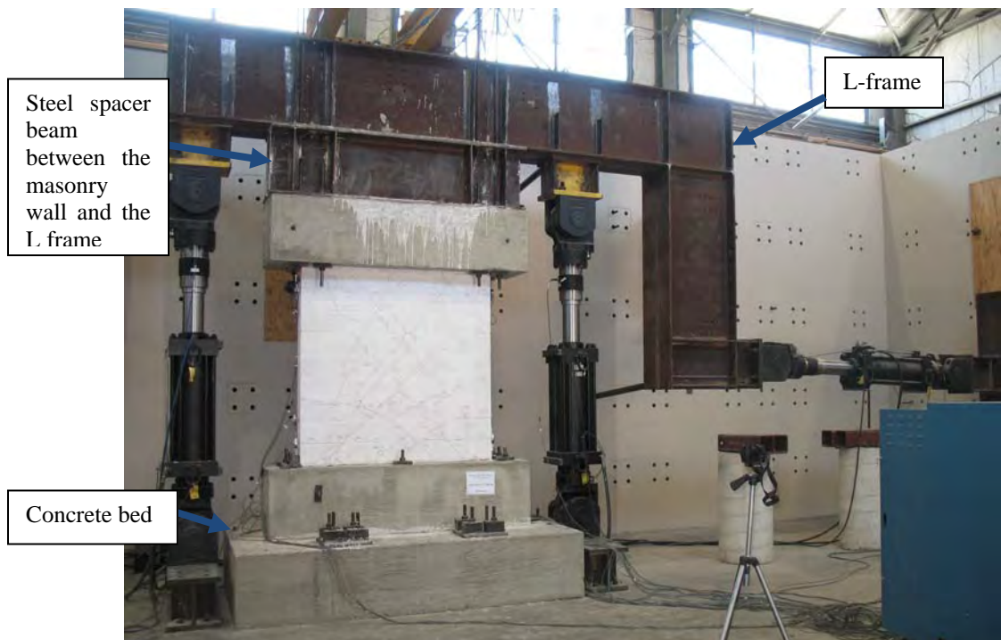
Figure 6.22 Test setup for the fix bottom – top rotation restrained masonry wall
