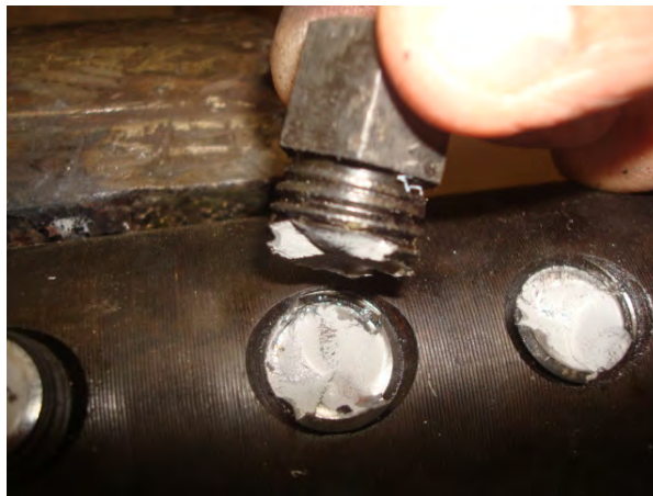
Figure I.31 Thread of the bolt broken
