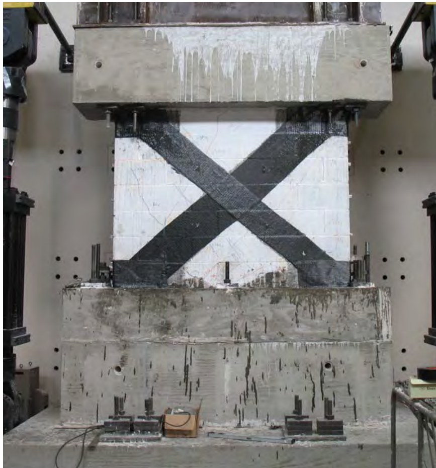
Figure 1.9 Masonry wall repaired by the concrete ring and diagonal ties of CFRP
