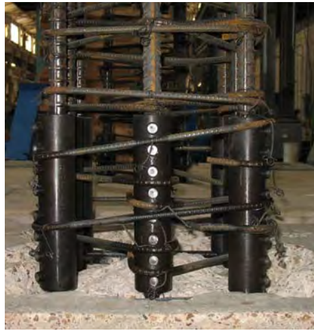
Figure 5.91 Long mechanical splices completely installed for specimen RC-2R-LMS
