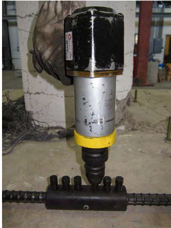
Figure 3.13 Torqueing the bolt into the mechanical splice
