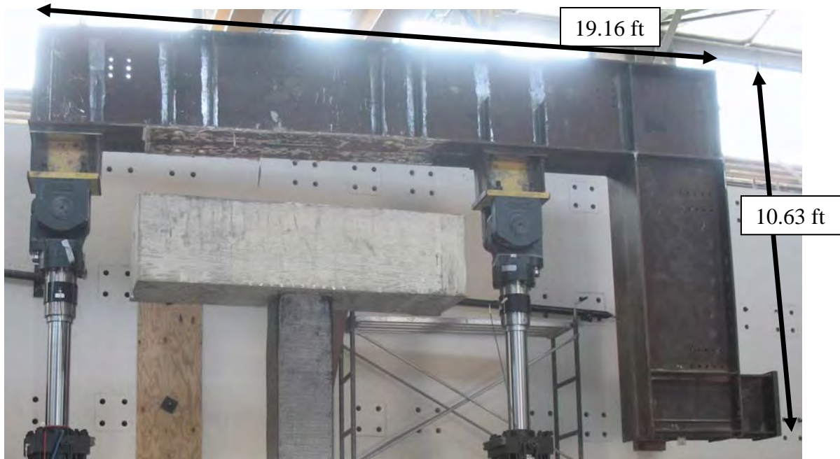
Figure 5.5 Steel L-Frame for loading columns
