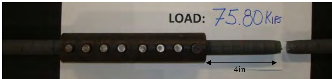
Figure I.6 MS-L1 failure pattern.
