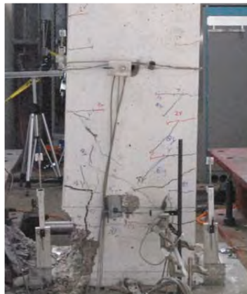
Figure 5.132 Flexural and shear cracks on east face of the specimen
