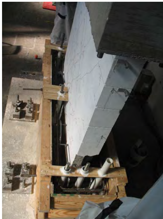
Figure D.3 Form for the concrete ring
